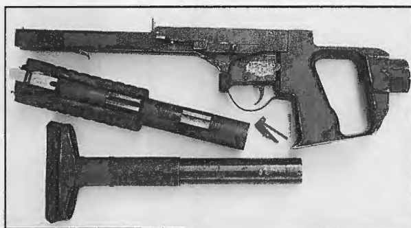
Left side view of field stripped M26A2 grenade launcher. Barrel stop must be removed to separate barrel assembly from receiver group. Note obliterated identification marks on receiver above trigger to disguise origin, which is most likely Cuba.
